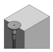
Mount the cap in the socket after removing the nailing plate.
